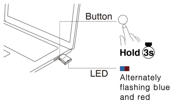
3. The headset and the WDD60 will pair automatically and the headset's LED indicator glows blue.
