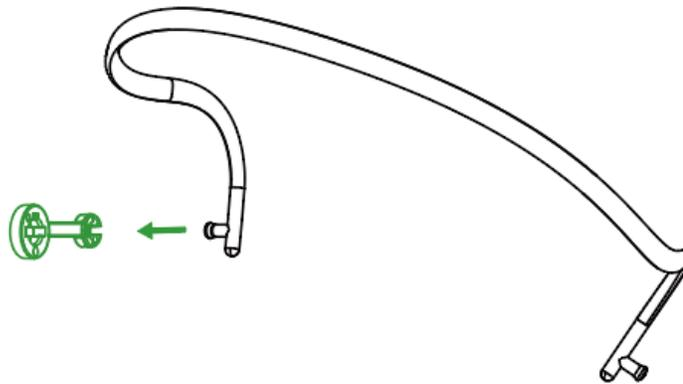
2. Install the connecting rod to the other end of the neckband.
