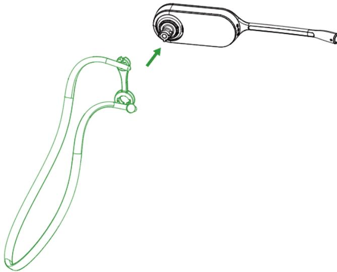
4. Choose the size of eartip that fits most comfortably. Align the eartip with the notch facing the microphone as shown. Press on to attach.
